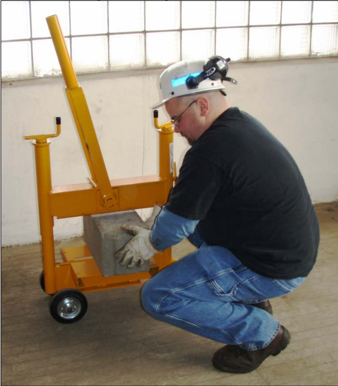
Figure 1: MPI Block Splitter - Block Placement
