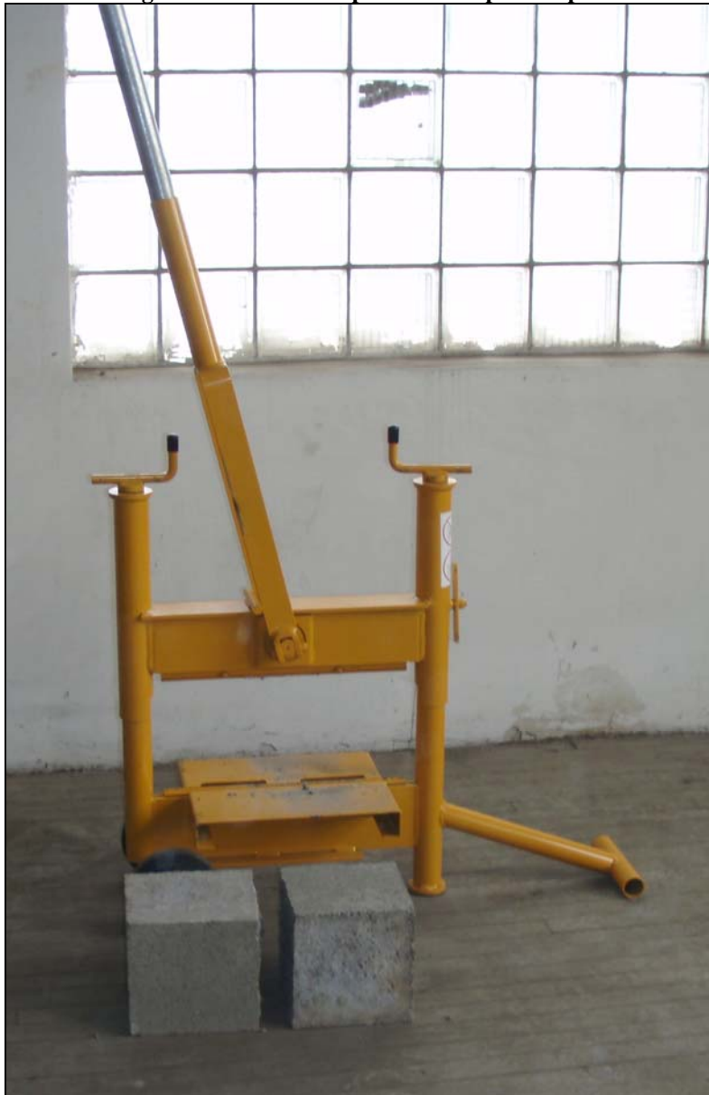
Figure 3: MPI Block Splitter - Completed Split
