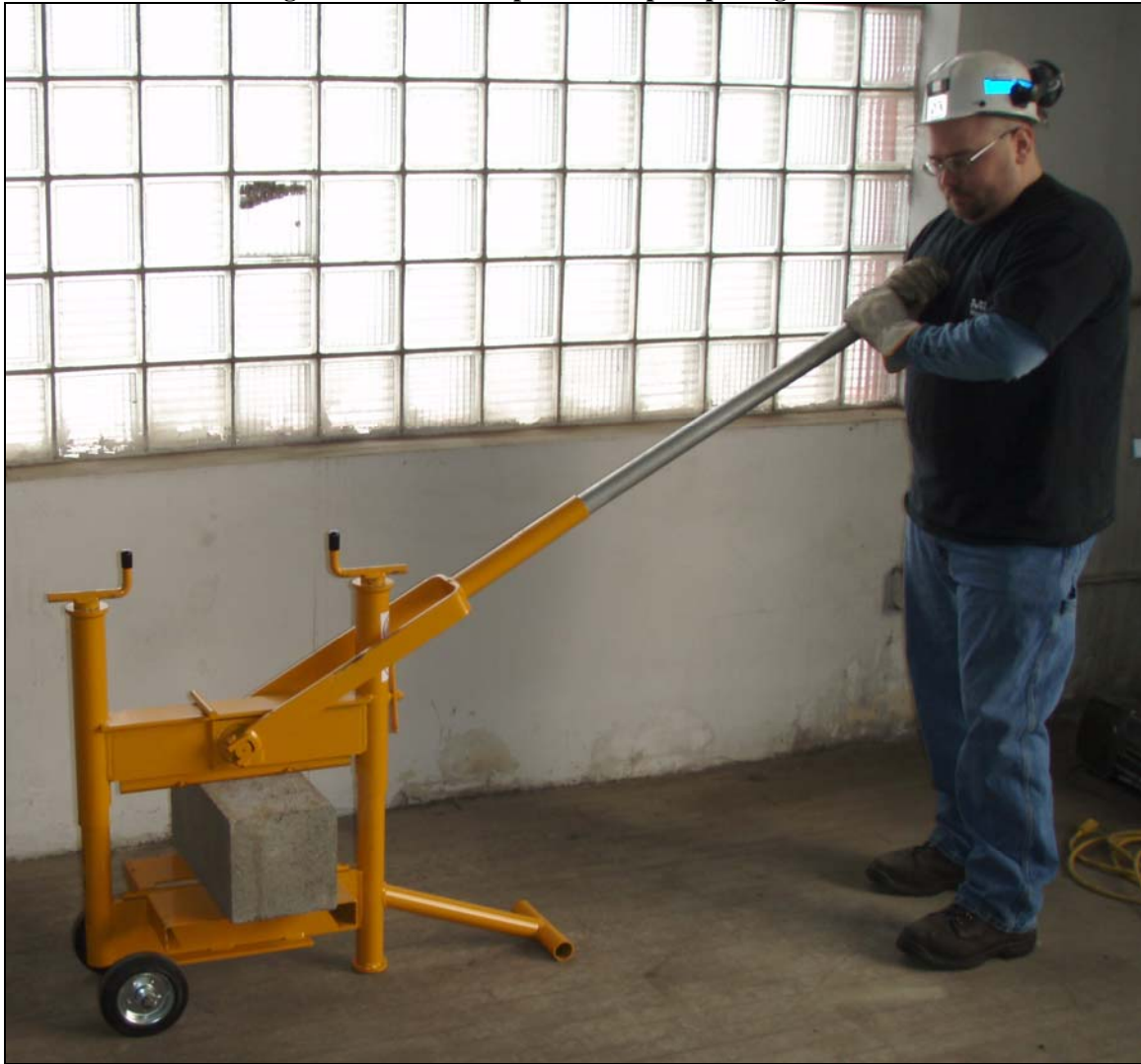
Figure 2: MPI Block Splitter - Proper Splitting Position
